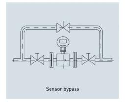
for sensor servicing. A Sensor bypass may be a also reasonable solution in the cases where, to dismantle the flow sensor from the piping, Liquid from a very long piping section would have to be discharged.
