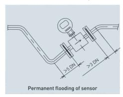
In piping systems where complete flooding of the piping cannot always be guaranteed, consider placing the sensor in a bottom pocket where full flooding is sure.
