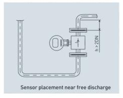
If the sensor is located near a free discharge point, such point shall be by at least 2 DN higher than the top part of the sensor.
