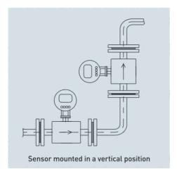
In the cases where the sensor is mounted in a vertical position, the flow direction shall always be upwards.
