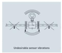
Make sure that the adjoining piping is clamped/supported as close to the sensor as possible, to prevent vibrations and damage to the sensor.
