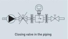
For the same reason, the sensor shall be always placed before the closing valve in the piping.
