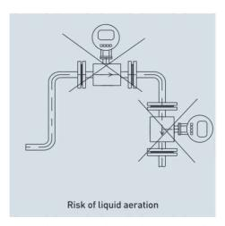
accumulate or develop in the sensor tube. Therefore the sensor shall never be placed in the upper Pocket of the piping or in a vertical piping section wher e the flow direction is downwards.
