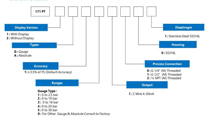
**NOTE:** Pressure Transmitter With Display only Provide the 4-20mA output.
