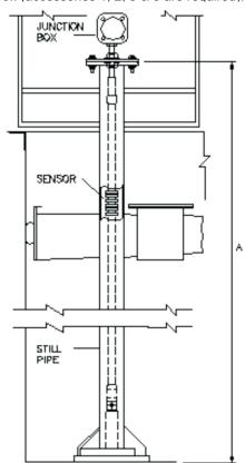
**Type 2** - On a mounting plate welded above a 2" still pipe \*which is welded inside the 8" manual gauging pipe. (accessories 1. 2. 4 & 5 are required).
