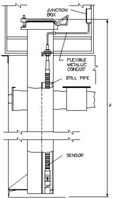
\* Still pipe extends to within 100 mm of tank bottom and has 2 rows of Ø 12.5 mm holes at 300 mm pitch. NOTE: Flange / Still pipe above 2" can be used with matching accessories.
