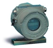
An accessory provided with STDT for remote indication of level, temperature, alarm status & diagnostics data. This is required when the float & tape type level gauge with STDT are mounted on top of the tank. The TSI provides indication of tank parameters at grid level. The 4 1/2" digit, 1/2" high, 7 segment LCD display unit is provided in the flameproof & weatherproof cast Aluminium enclosure, with accessories suitable for pipe mounting.
