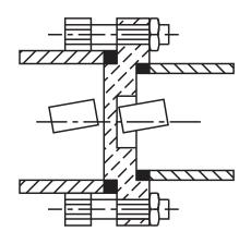
The float movement of the level switch is transmitted through a solid non magnetic wall by the repulsion of like magnetic poles. This ensures that the float magnet imparts a snap action to the electric or pneumatic switch elements. `S.B.E.M.' level switches are absolutely leak proof & not subject to material fatigue due to gland less design.
