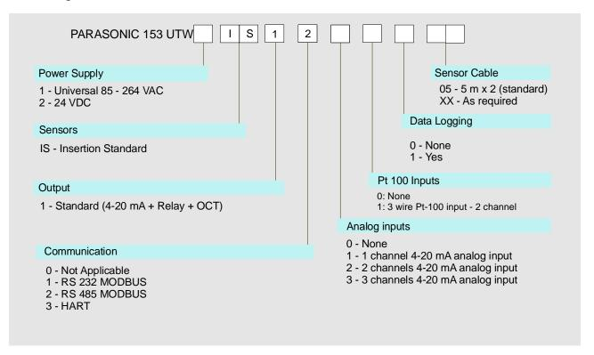
Example of Model Code Selection for Wall mounted Ultrasonic Flow Meter with Tapped Insertion Sensors:
